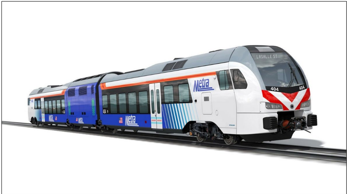
Figure 5 – 2-Car BEMU Rail Vehicle Developed for Chicago Metra
